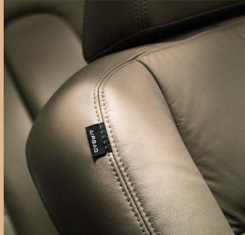
The new side airbag supplemental restraint system enhances front-passenger protection in certain side-impact collisions.
